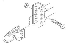
Figure 8-6. Combination Hitch Installation
